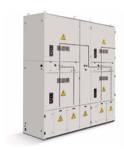
In DC Traction Substations one disconnector or load break switch is normally installed downstream each High Speed Circuit Breaker thus allowing, in case of failure, to isolate the circuit breaker granting the safety of the system. The configuration is then completed by a bypass or parallel disconnector switch connecting two feeders and allowing to grant the service continuity in case of failure of one circuit breaker: this disconnector is normally on-load and motorised for remote control.
