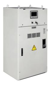
In a DC Traction System the return circuit (negative) shall usually have high insulation level against earth to limit stray currents phenomena. In case of dangerous overvoltages, the return circuit shall be short circuited to earth. For this purpose a voltage limiting device shall be installed on each negative path.
